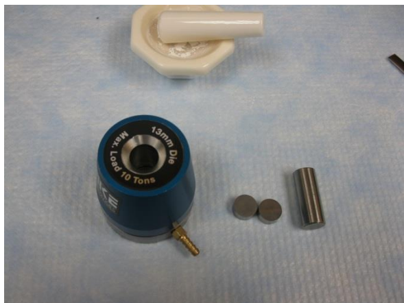
3). Transferred the mixed sample to a pellet-forming die
