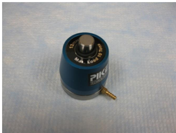
4). Assembled the pellet-forming die.
