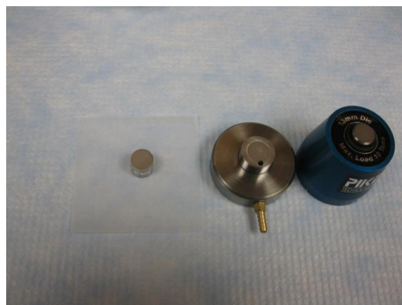
6). Took out the pellet from the pellet-forming die.
