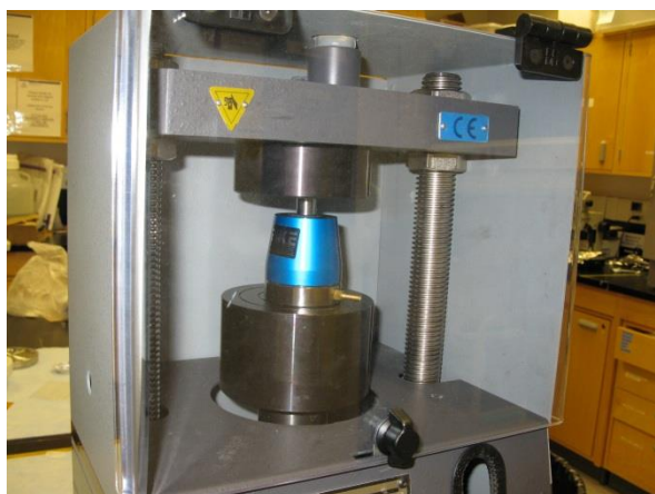
5). A force of approximately 10000 pounds is applied for a few seconds to form pellets.
