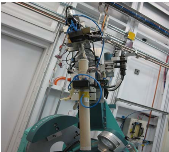
Figure 1.2 Psi-8 diffractometer detector arm with analyser setup.
